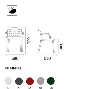
Net weight Gross weight Max. Stacking Packaging Shipment Details (kg)(kg)201 216 pcs. 40' 456 pcs. 4,60 5,40 40HC : 600 pcs. cardboard package 100cbm :784 pcs. 715x610x947mm / 0,41m<sup>3</sup>
