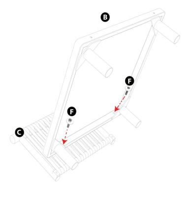
Fix the modules to each other with to help of connection part for corner structure.
